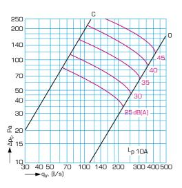
EHC without or with connection box (connection alternative SIDE = A and OVER/UNDER =C).
